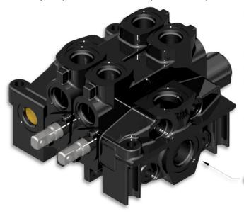
Once the valve outlet section is installed an unobstructed path back to tank will need to be plumbed to complete the circuit. Any secondary control valves plumbed into the circuit, between the VG20 control valve and tank, will need to be open center and have its own built-in relief valve set at or below the pressure setting of the VG20 control valve.
