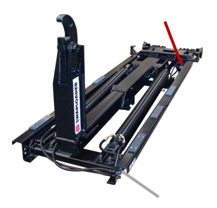
Serial Number Tag is located at the front driver side of the hoist (gray arrow on first picture).
